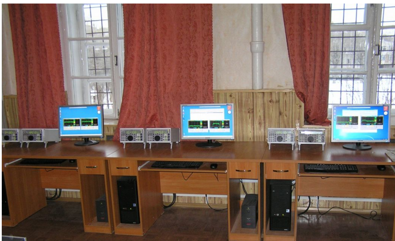
Operators' working places with two receivers “Galaktika-M” and demodulators W-CODE
