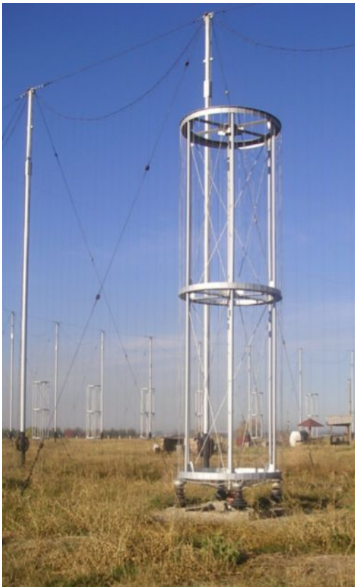
General view of antenna elements of direction finding AFS of "Krug-M-A" product
