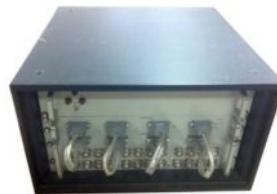
Matrix switch 40 inputs and 3 outputs 4-channel receiver CRPU-1k/4t
