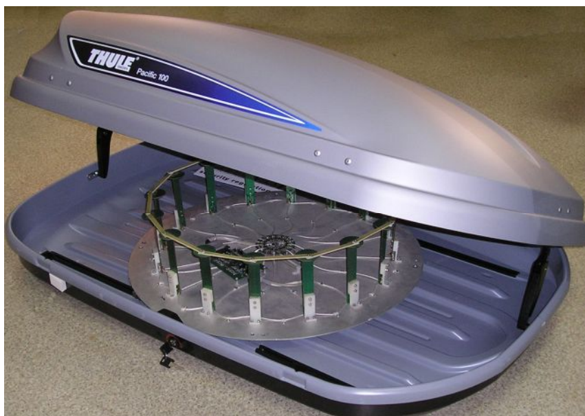
View of AFS of direction finder “Pauchok-M” and receiver “Филин-VU/DF-02”
