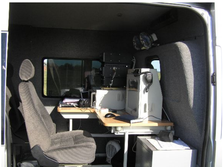
Operator's position of «Barvinok-M» station
