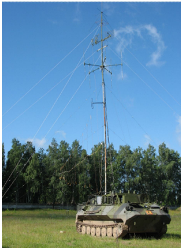
"Barvinok-OP" station mounted on the APC
