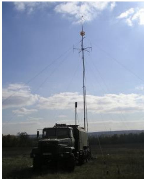
"Barvinok-OP" station mounted on the «KRAZ» truck
