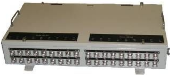
Unit of wideband input devices and switching
