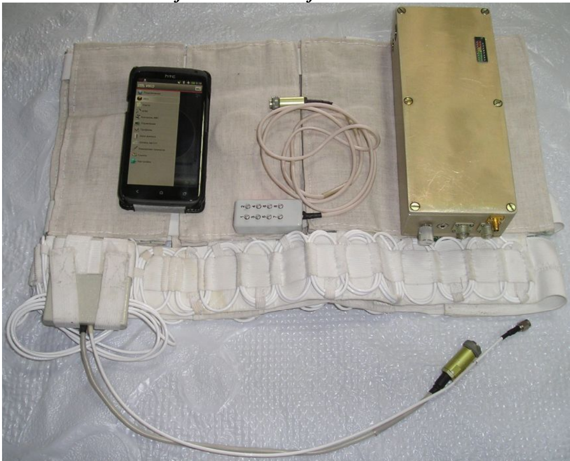
View of radio direction finder “Philin-A”
