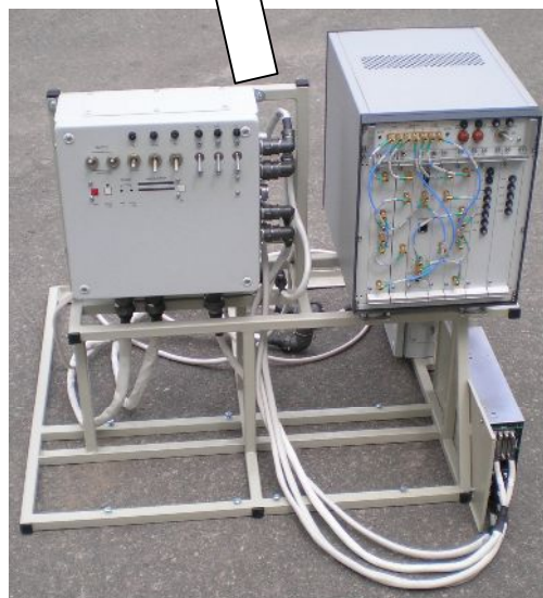
Two two-channel receivers of detector-direction finder and executive direction finder
