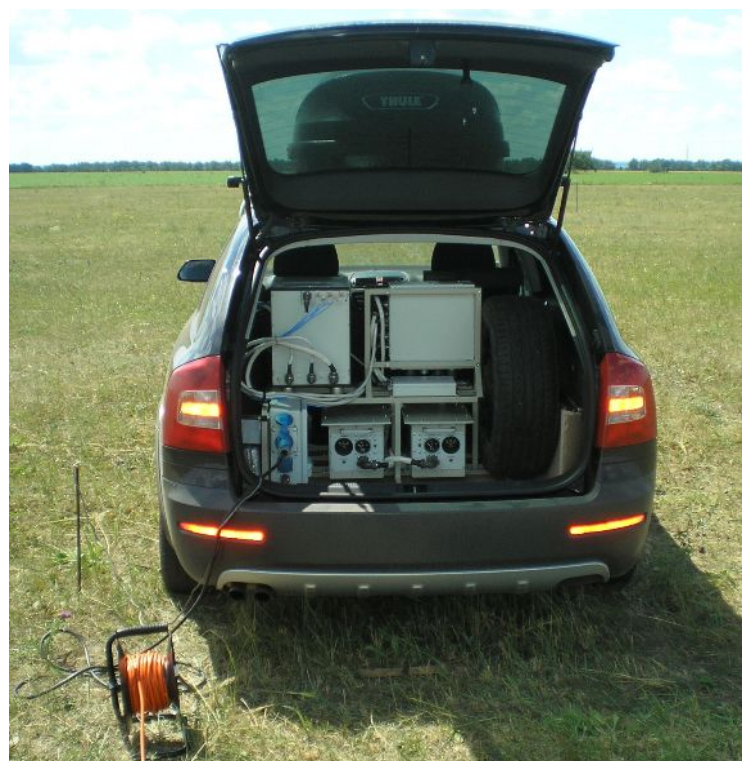
Arrangement of "SCORPION-M" equipment inside a vehicle
