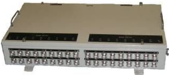
Unit of wideband input devices and switching
